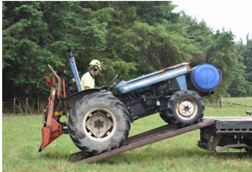
Small-scale trial using farm-based machinery ... a 45-hp tractor with 4-tonne pulling capacity.
