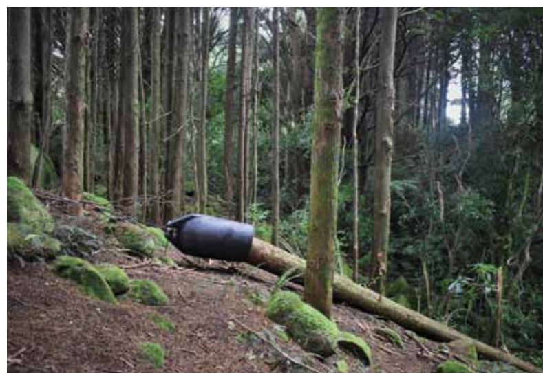
Figure 5: The D.I.Y. skidding cone proved its worth. The nose cone helped avoid snagging the logs on rocks, roots, humps and stumps, and minimised soil disturbance and damage to the forest
