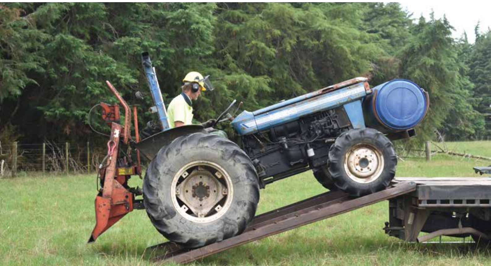
Figure 3: European-style forestry equipment – a 45-horsepower tractor with a PTO-driven winch on the 3-point linkage and a 4-tonne pulling capacity
