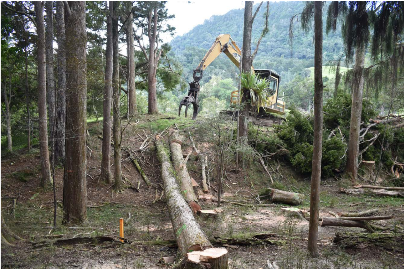
Grapple diggers are extremely versatile machines but tracked machines should not enter the forest. They need to stay on tracks or work from paddock edges.
