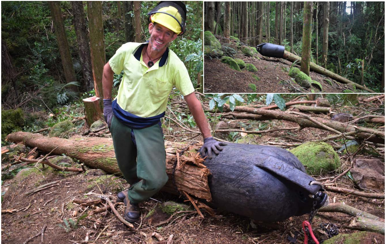
The ever-ingenious Li Legler, with his skidding cone fashioned out of a buoy from a mussel-farm. Inset: The D.I.Y. skidding cone enabled tōtara logs to be winched out of a steep and rocky gulley, from the paddock edge and with a small tractor-mounted winch. The choker-chain on the log passes through a hole in the 'nose cone' and is then hooked to the wire rope.
