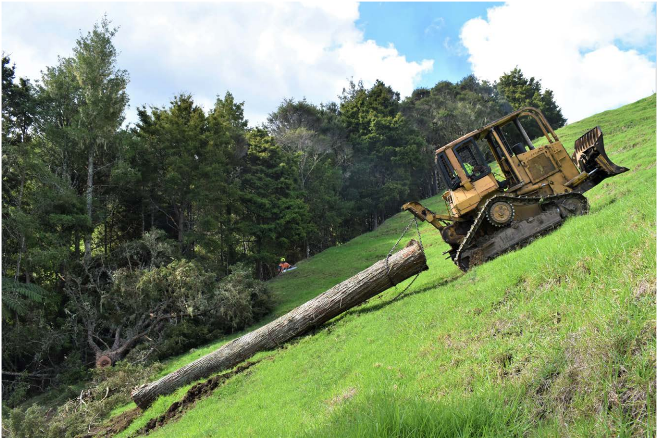
A D4 TSK skidder is a powerful and safe machine capable of extracting large logs and working in steep terrain.
