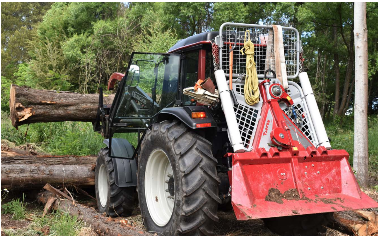
Roger May has an excellent tractor-logging set up comprising a 4WD Valtra tractor with a front-end loader and 6.5-tonne Tajfun skidding winch that can be operated from a remote controller on the belt. This enables the operator to see the log at all times.
