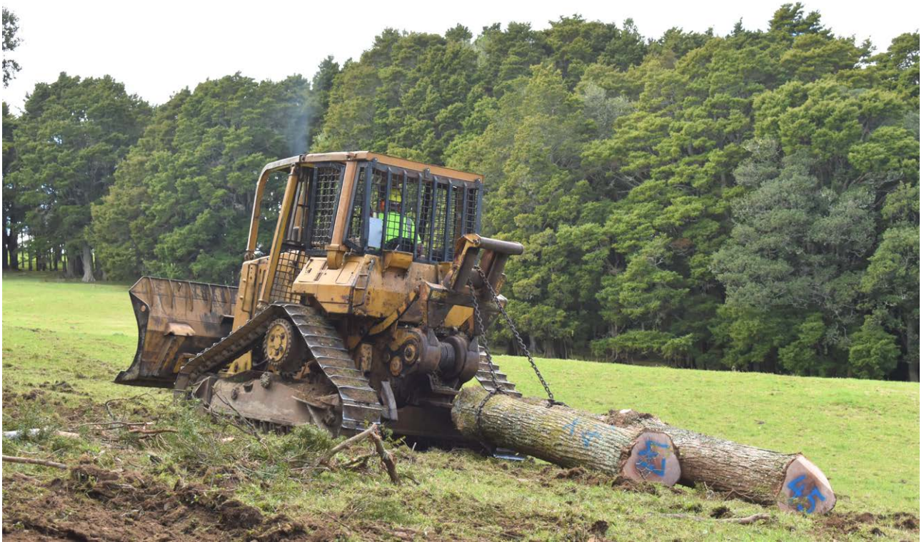
Tracked skidders are built for the job, but they are a slow and expensive way to skid a few small logs over long distances.
