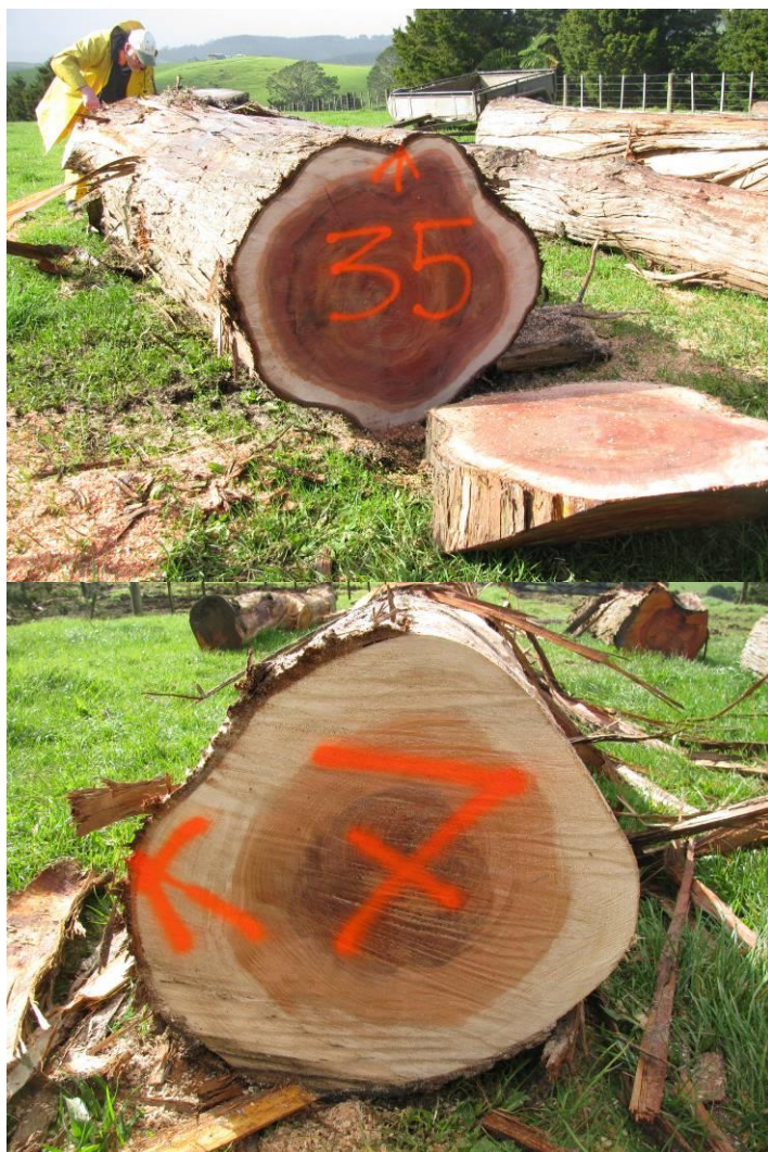
Figure 8: The above cross-sectional views of logs from farm-totara trees show varying amounts of heartwood. Log number 35 displays the deep reddish-brown colour traditionally associated with heart-totara. In contrast, log number 7 (a top log in this case), shows the more typical characteristics of younger stems; a larger proportion of sapwood, and often an in-between area of insipient heart, and a small core of darker heartwood.
