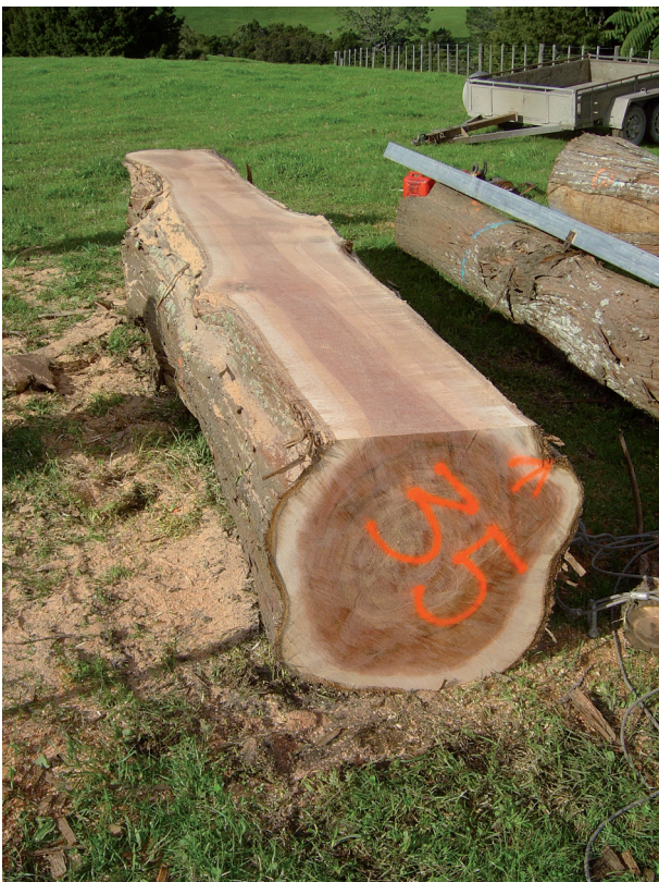
FIGURE 5: An example of a farm-grown totara log. The darker wood in the centre is durable transition wood and heartwood; the lighter area towards the bark is sapwood.
