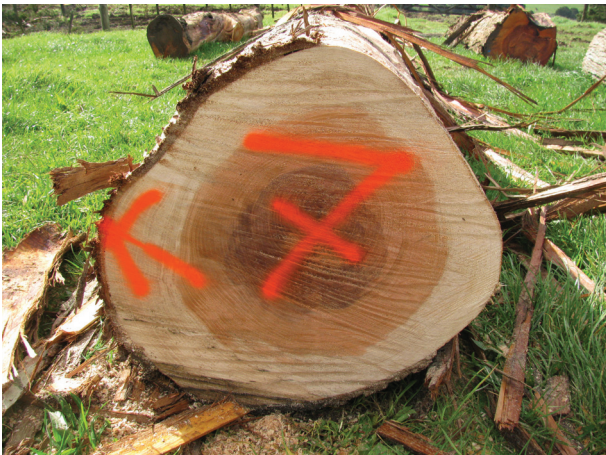
FIGURE 2: The above cross-sectional views of logs from farm-totara trees show varying amounts of heartwood. Log number 35 displays the deep reddish-brown colour traditionally associated with heart-totara. In contrast, log number 7 (a top log in this case), shows the more typical characteristics of younger stems; a larger proportion of sapwood, and often an in-between area of incipient heart, and a small core of heartwood.
