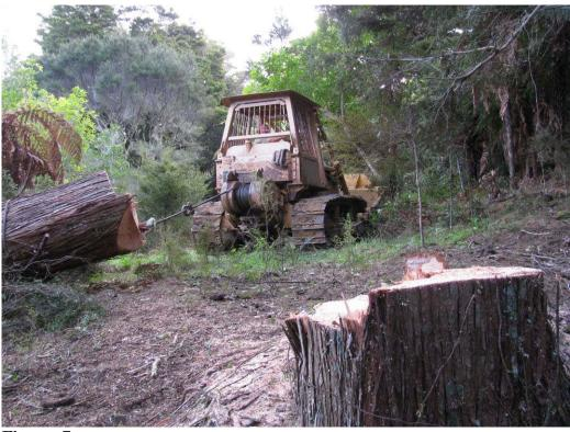
Figure: 7 John McGee winches a farm-totara log to a farm track with a D6 Bulldozer.
