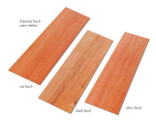
Silver beech steam-bends easily. Compared with other native beeches, it is lighter and more easily worked, but less durable. Neither heartwood nor sapwood of silver beech is durable in high hazard situations, so it is unsuitable for outdoor applications. However, the timber can be used for interior and indoor furniture applications without the need for treatment.
