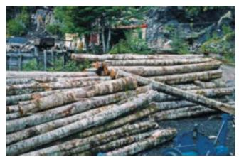
Beech timber was used extensively in both gold and coal mines as mine props as the timber was not only strong but "talked" (creaked) as it was compressed, providing a warning to miners of possible movement in the roof of the mine.
