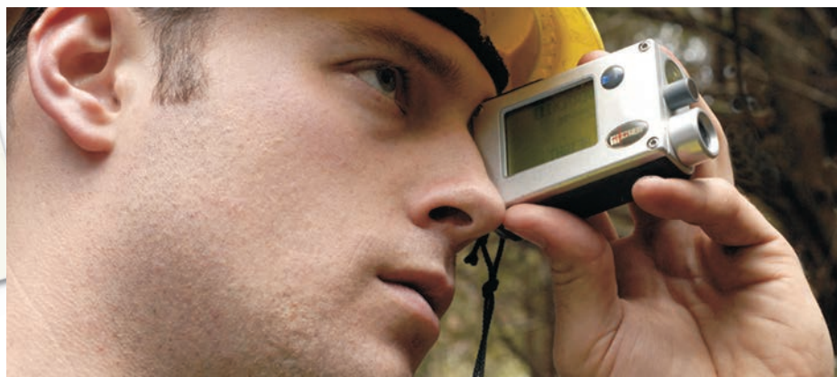
A Vertex Hypsometer is used to accurately establish Permanent Sample Plots and to measure tree heights.
